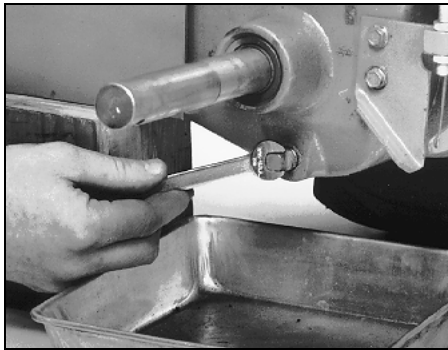
Figure 5-4: Remove drain plug to drain transmission gear oil (also remove oil fill plug and oil level check plug).
